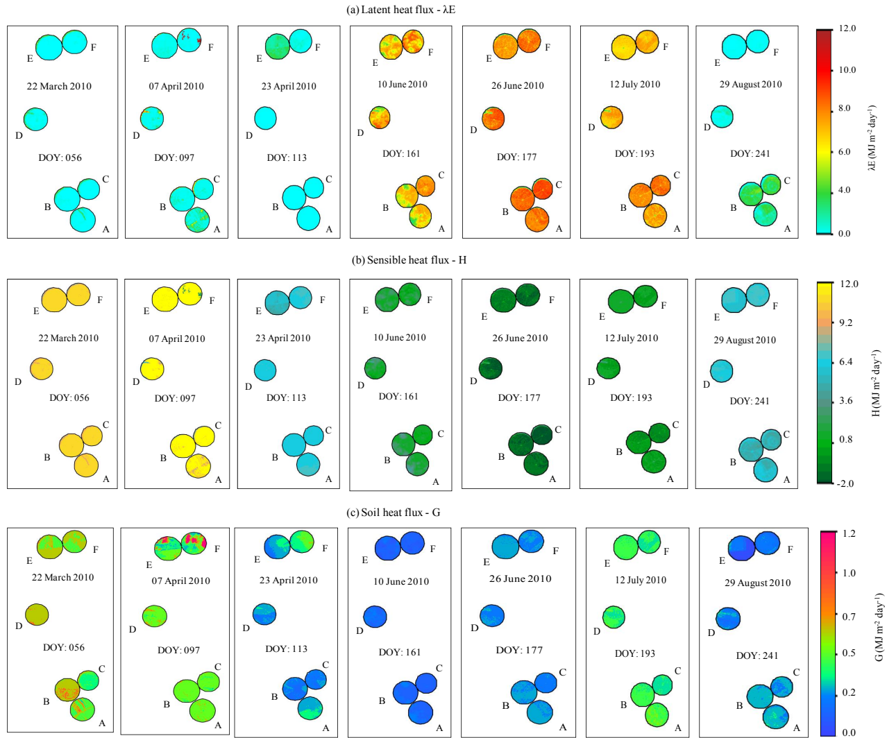
Figure 5. Spatial distribution of the daily values of the energy fluxes in the corn crop central pivots in Bonança farm, Northwestern side of São Paulo state, Southeast of Brazil, for each day of the year (DOY), involving different thermohydrological conditions along the growing seasons. (a) latent heat flux ( \lambda E ); (b) sensible heat flux ( H ); and soil heat flux ( G ).
